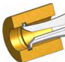
Schneide R0,1 mm blade R0.1 mm
